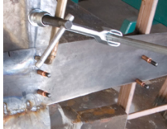
Möbius, with clecos attaching it to the frame
