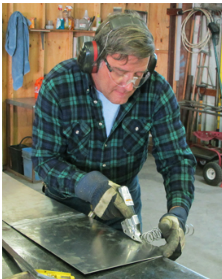
Kevin cutting aluminum with pneumatic shears
