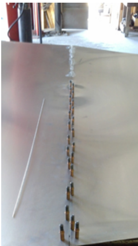
Two panels of The Seed held by cleco fasteners
